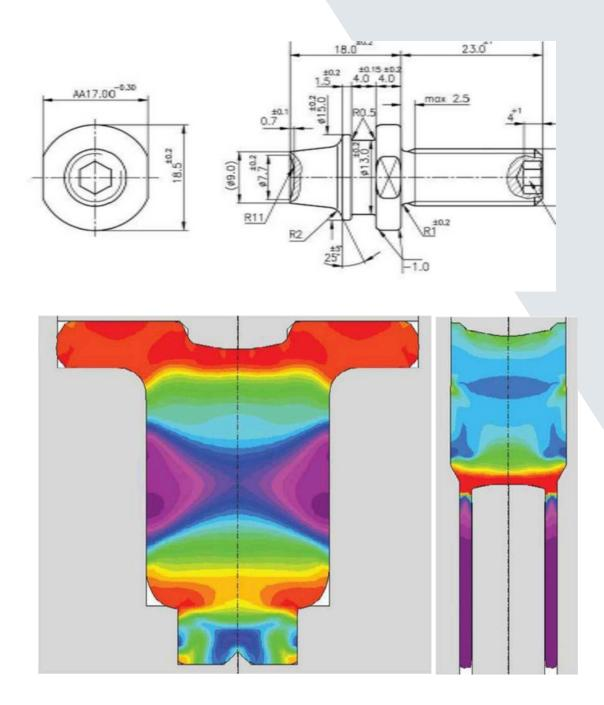
Teknoform uses simulations in cold forging of special fasteners in order to eliminate mistakes before the tools are made and production begins. Ability to see maximization of tool life and accurate calculation of loads required for cold forming. It also optimizes the tool plans and production drawing with fast and efficient way. Encountering of overloaded condition to tools is blocked and can be extended tool life.
