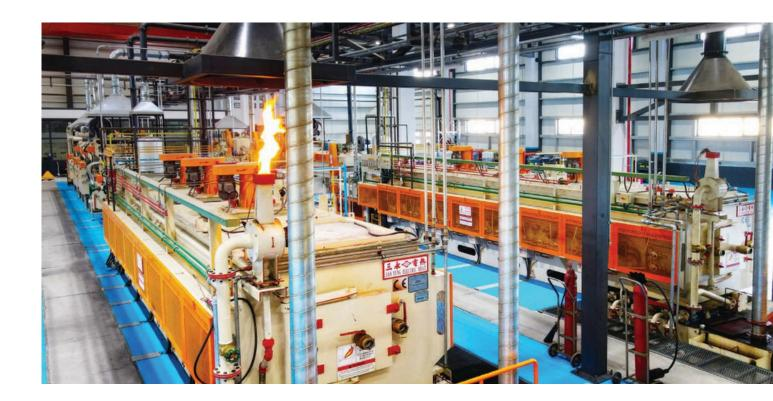
Our heat treatment furnaces have 750 kg per hour production capacity, computer controlled, automatic loading, automatic oxygen, carbon control and dephosphating units are included in the system, also available with % 100 detection systems agglomeration. It is also supported by the latest technology of hardness measurements and reviewing internal structure of products.
